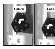
Turn the handle clockwise to lock the stop in position. The handle only requires a rotation of 90 degrees from locked to unlocked. Lift and rotate the adjustable handle to position it in the proper quadrant.
