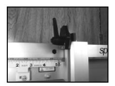
Install the stop/spacers in the opening at the end of the track. The knife carriage must be removed out of the top of the vertical tracks to install the bottom stops.
