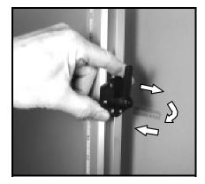
Lift slightly and rotate the spacer block to change the spacing. The block will snap down into the new position. The following spaces are available:
